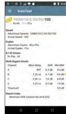
Cabling SNR measurement validates Multi-Gig links
